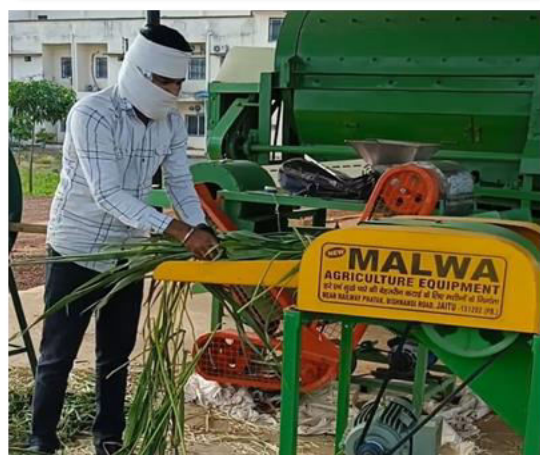
Fig.1 View of the power operated chaff cutter while in operation
